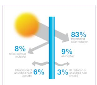
For example, 3mm clear glass: 83% of solar radiation is transmitted, 8% reflected and 9% is absorbed. 3% is then radiated inside and 6% outside.
