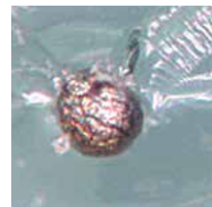
Nickel sulphide inclusions found on fracture surfaces of glass that failed by "spontaneous breakage".
