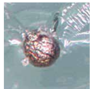
Nickel sulphide inclusions found on fracture surfaces of glass that failed by "spontaneous breakage".
